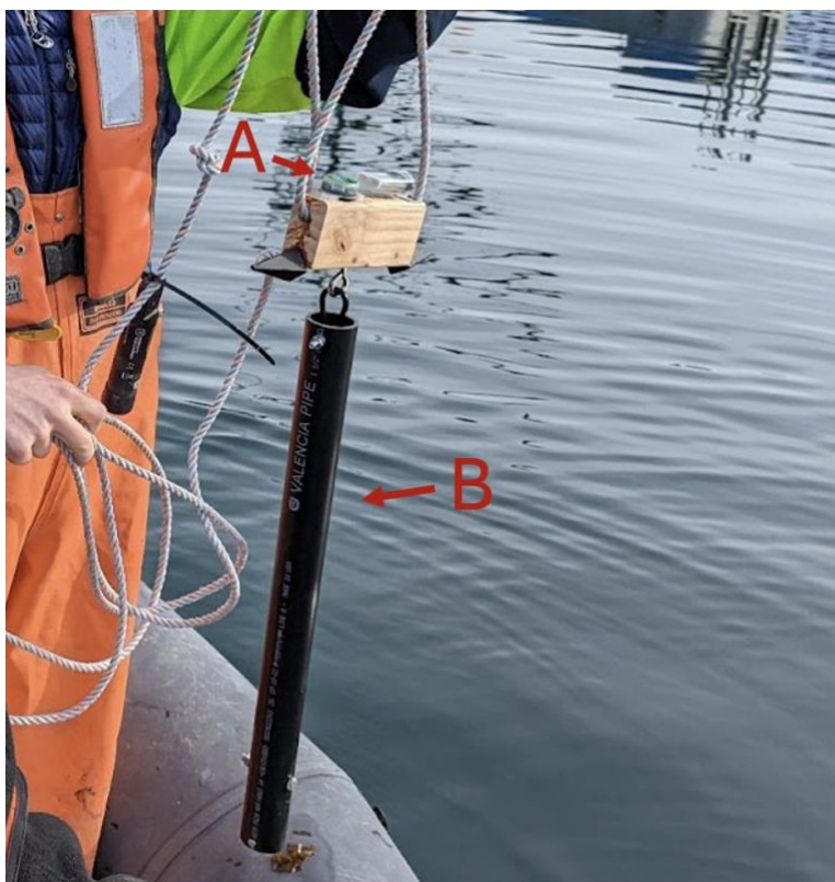
Figure 3. Picture of the logger array system deployed at five kelp farm sites in Alaska between April and June of 2023. A) HOBO MX and B) HOBO Pendant G in a PVC casing. The system was fixed to a sinking line.
