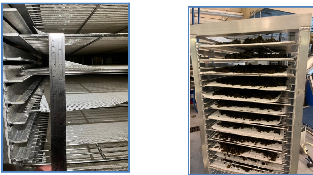
Figure 1. Dryer cart and shelving rack unit showing the rack spacing (left) and the cart loaded with the maximum 24 racks of kelp (right).
