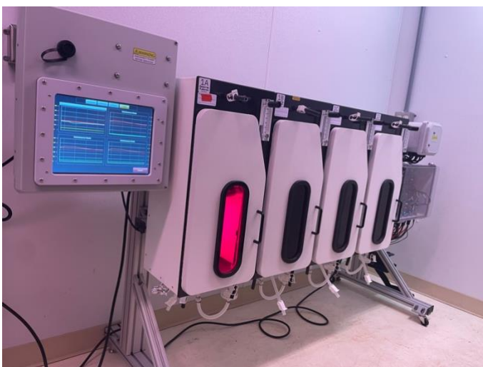
Industrial Plankton Seaweed Bioreactor.
