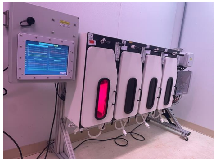
Industrial Plankton Seaweed Bioreactor. Each module houses one, 2 liter culture chamber with
