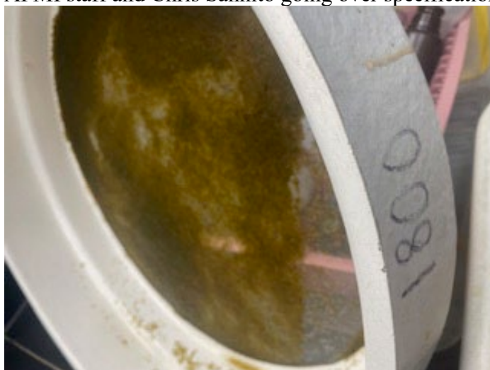
1800-micron screen holding the slurry that passed through the 2400 screen
