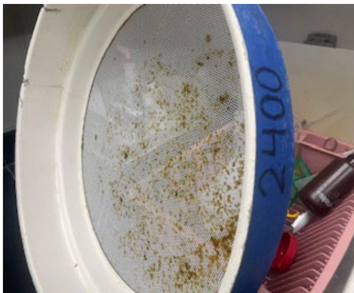
2400-screen holding some of the slurry flakes that did not impact nozzles
