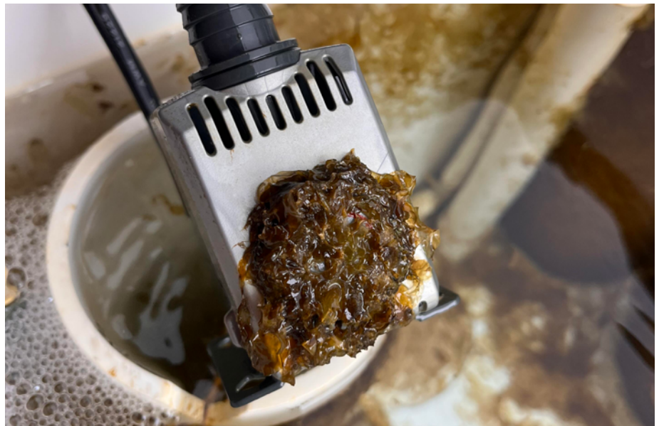
This water pump from a nursery tank is clogged with sporophytes. The intake should be cleared out using a clean brush or paper towel.
