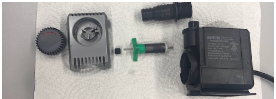
Take apart every possible part of your tank and nursery system to clean it entirely. The water pumps can be broken down into six parts for thorough cleaning.
