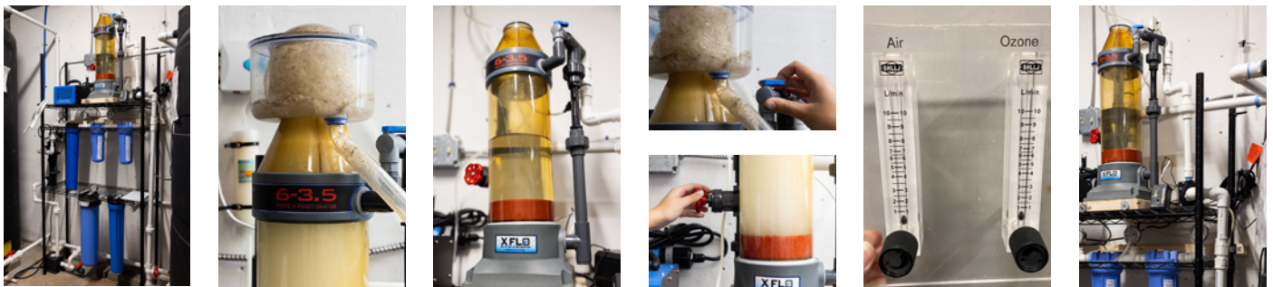
From left to right: Positioning, waste collection, adjustments, top: water input volume, bottom: output valve, ozone/aeration control, and pump compatibility
