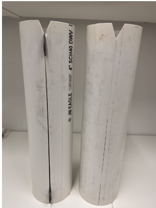
Place washers in the spool slit to prop it open during cleaning and sterilization.
