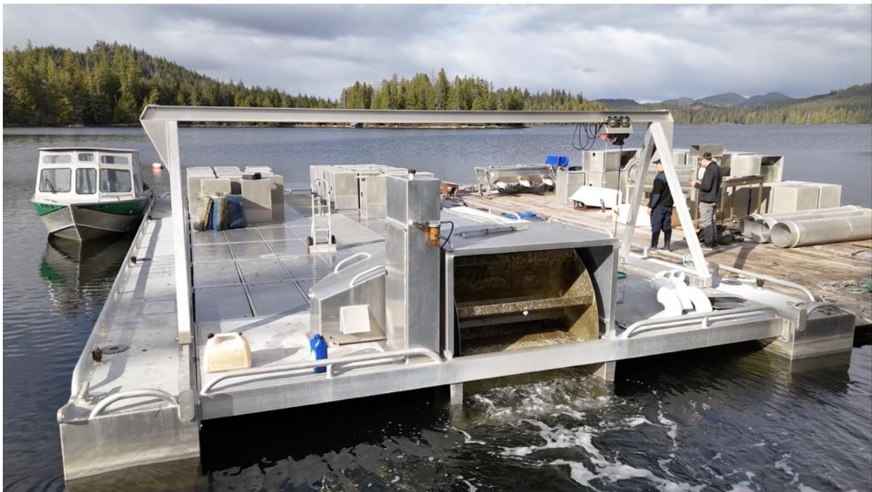
A FLUPSY owned by a member of the AOC, growing oyster seed to desired sizes. Jonny Antoni photo.
